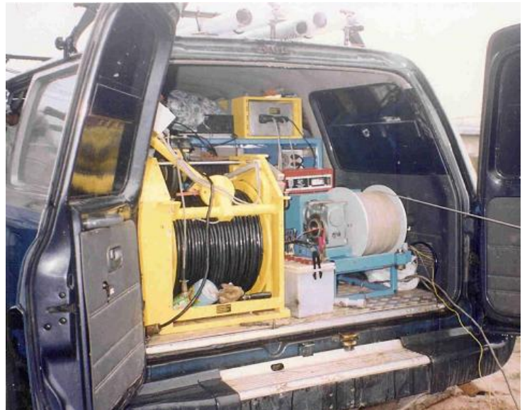
Plate 1. The RG PC Logger II™ Unit mounted on sports utility vehicle used for borehole loggings utilized for the study.
